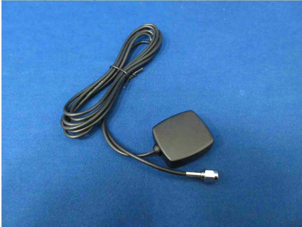
(9) EUT Photo (GPS Antenna)
