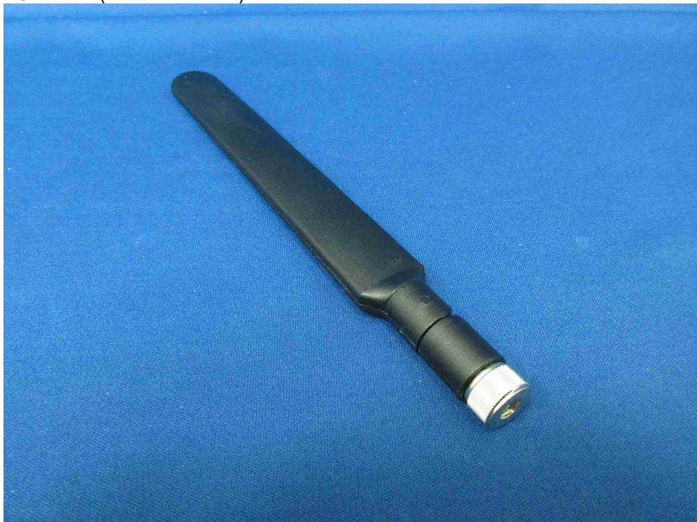
(8) EUT Photo (WWAN Antenna)
