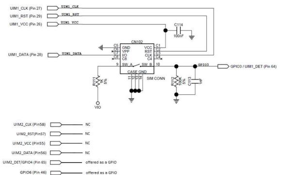
Figure 22. Single USIM Application (1 USIM Slot and 1 USIM Connector)
