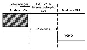
Figure 17. Power OFF Sequence for PWR\_ON\_N, VGPIO
