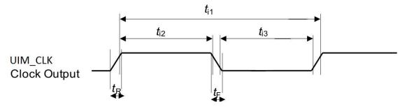
Figure 6. UIMx Timing Waveform
