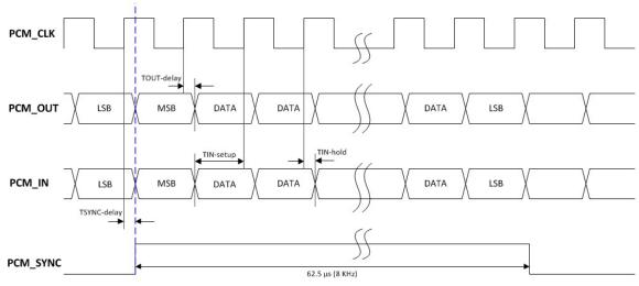
Figure 8. PCM Timing Waveform
