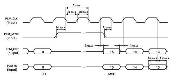
Figure 10. PCM Master Mode Timing
