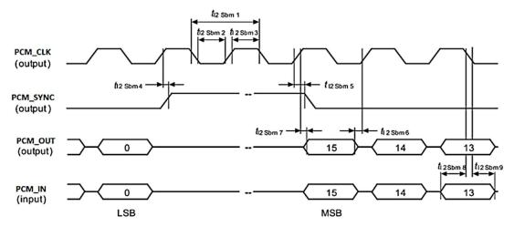
Figure 9. PCM Master Mode Timing
