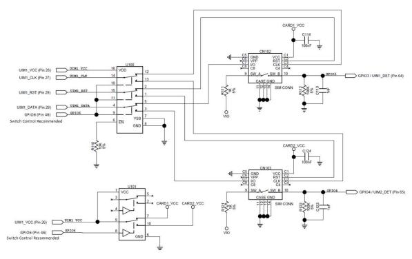
Figure 23. Dual SIM Single Standby Application (1 USIM Slot and 2 USIM Connectors)
