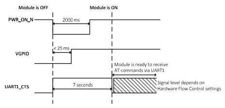
Figure 16. PWR\_ON\_N Sequence with VGPIO Information
