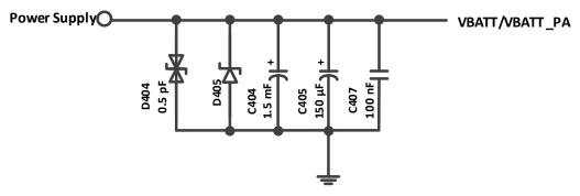
Figure 19. Voltage Limiter Example
