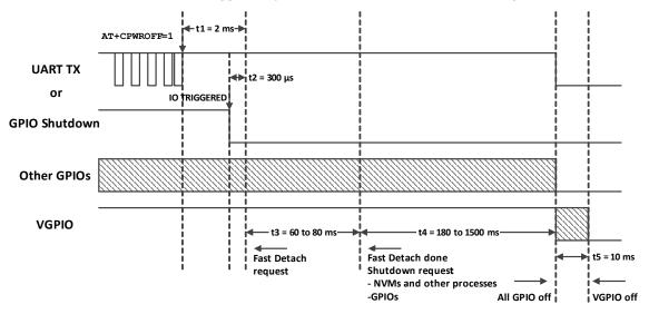
Figure 18. Fast Shutdown Power OFF Sequence
