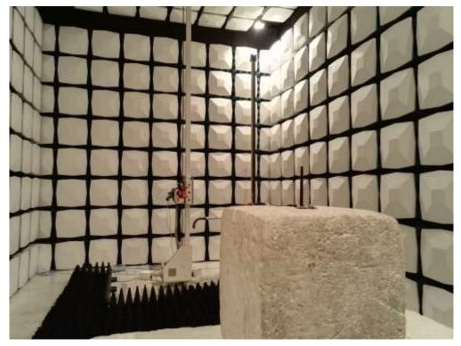
Description: Substitution Antenna for EIRP Test
