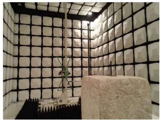
Description: Substitution Antenna for ERP Test
