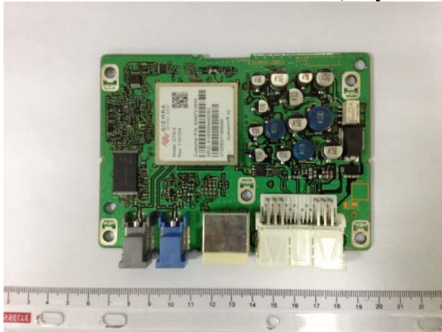
PCB, with module & RF Connections (Gray=GPS, Blue=CDMA)
