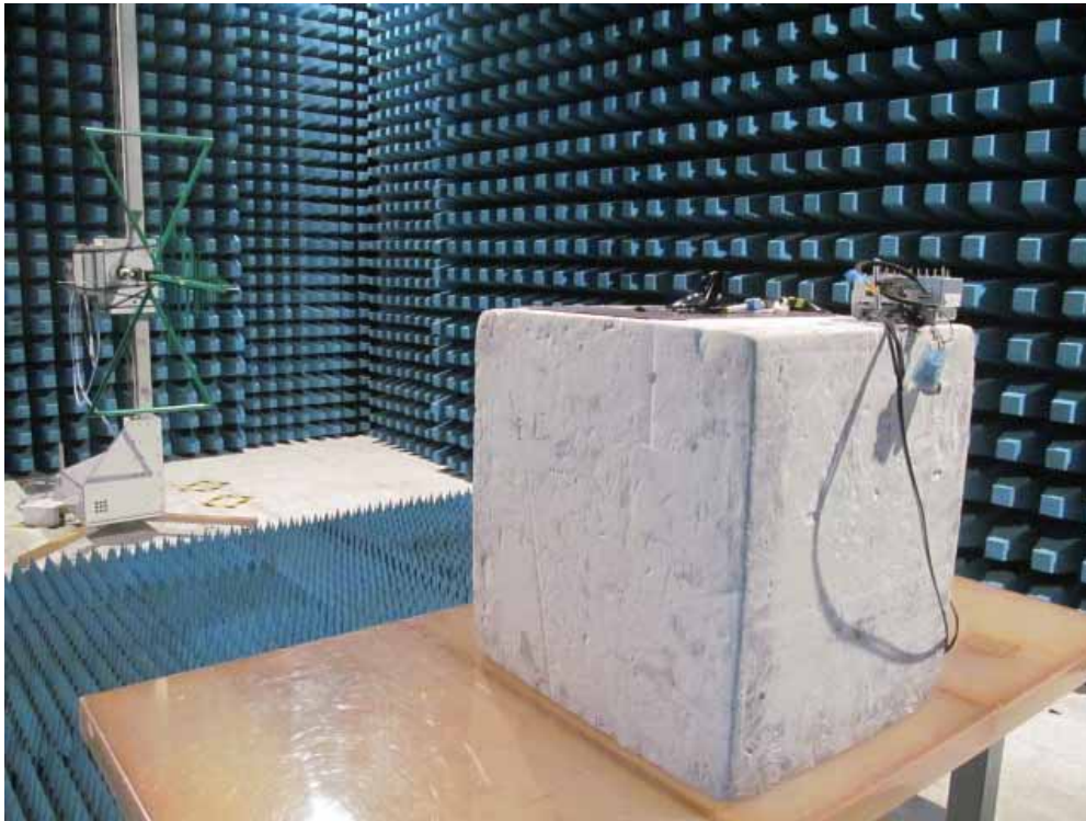
Description: ERP Test Setup with Antenna #2
