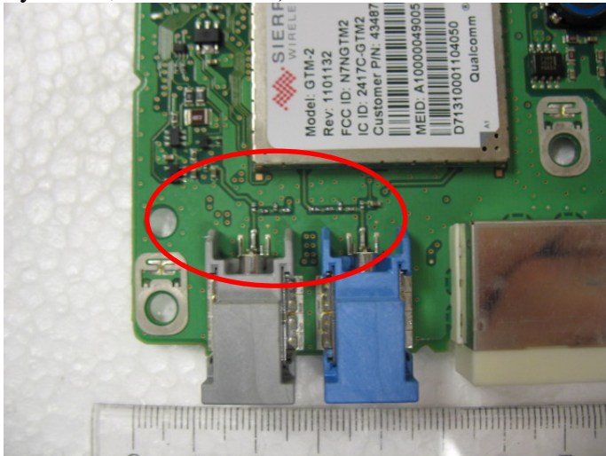
PCB, Antenna circuit details - Deviation from Module Certification (Gray= GPS, Blue=CDMA)
