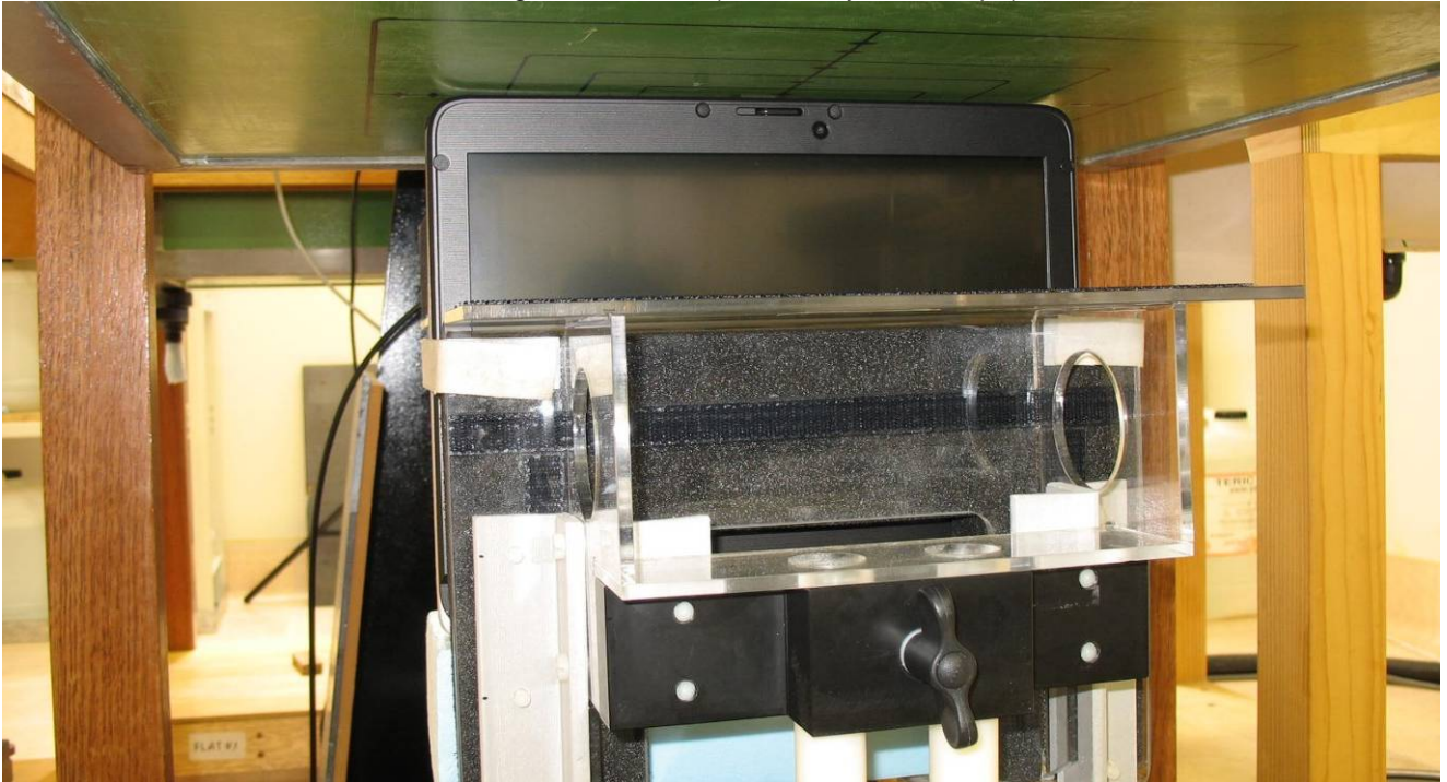
Photo No. 12: Edge On Position (Secondary Landscape) Antenna IN
