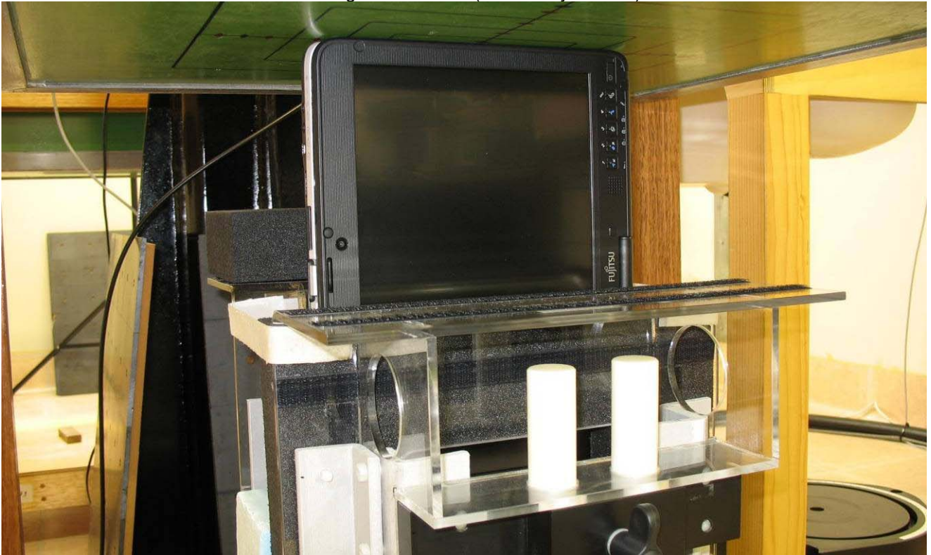
Photo No. 8: Edge On Position (Secondary Portrait) Antenna IN
