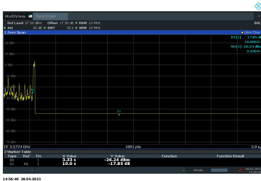
[Step 1] Configure SAS granted CBSD to operate at frequency 3670-3690MHz and power level 20 dBm/MHz
