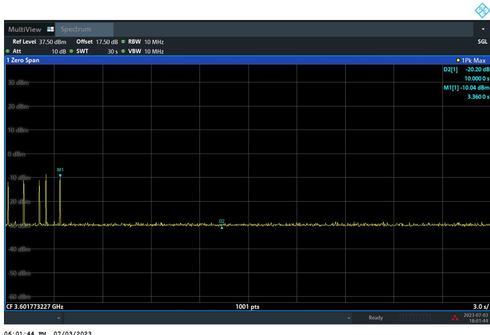
[Step 5] Configure SAS granted CBSD to operate at frequency 3670-3690 MHz & power level 7 dBm/MHz
