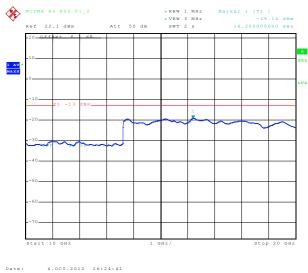
8.2.1.7 Out of Band Emissions at Antenna Terminals WCDMA B5, Middle channel, 836.4 MHz, 2 Hz to 1 GHz
