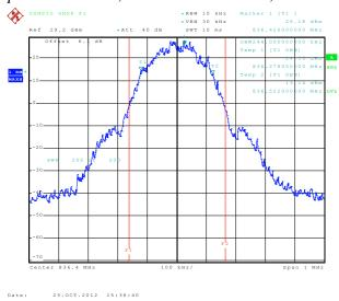
7.2.2.2 8-PSK Occupied Bandwidth, Cell Middle channel, 836.4 MHz, 99% bandwidth
