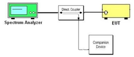
The companion device is certified CBRS (FCC ID: S9GQ710US00). Where the Companion Device connection with EUT is by radiated method.
