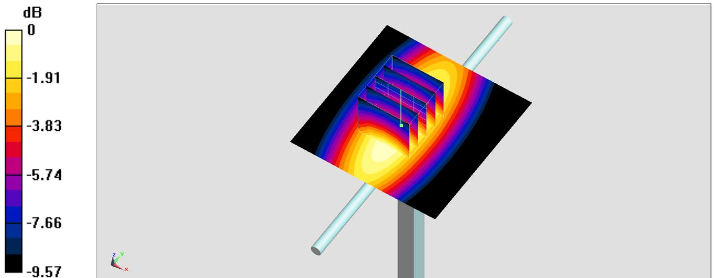
0 dB =  $2.64 \text{ W/kg} = 4.22 \text{ dBW/kg}$
