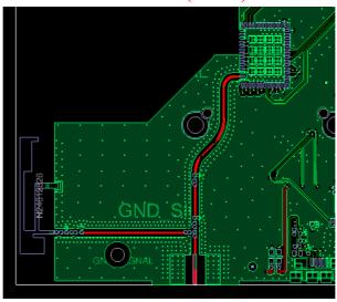
==RF traces @ LAYER 2 reference to Layer 1, 3, width: 9mil Please adjust the trace width to fit 50 ohm. (in Purple)
