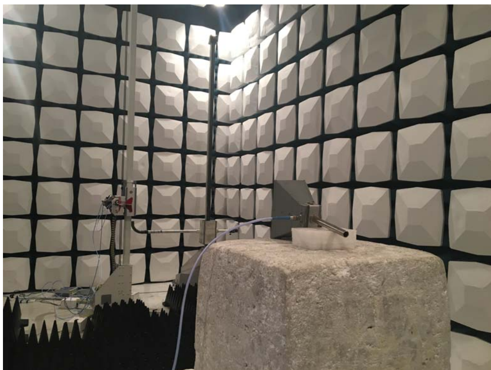
Description: Substitution Antenna for EIRP Test
