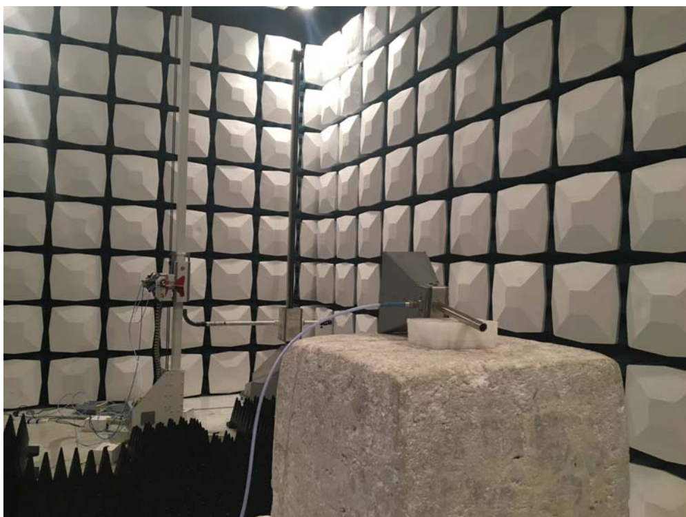
Description: Substitution Antenna for EIRP Test
