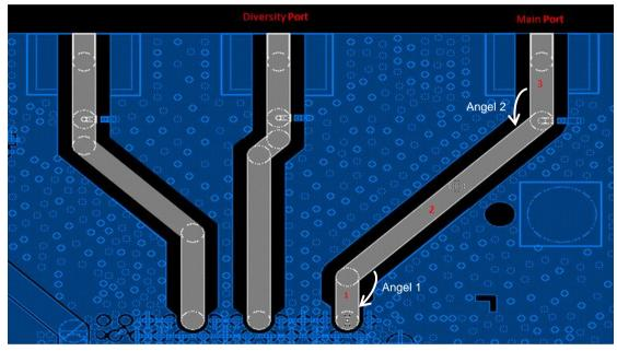
Figure 7. The definition of RF trace in the AR7552 CCB
