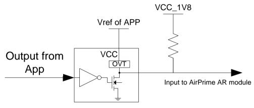
Figure 5. AirPrime AR7552 Input Reference Circuit
