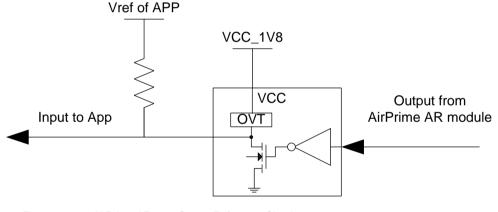
Figure 6. AirPrime AR7552 Output Reference Circuit
