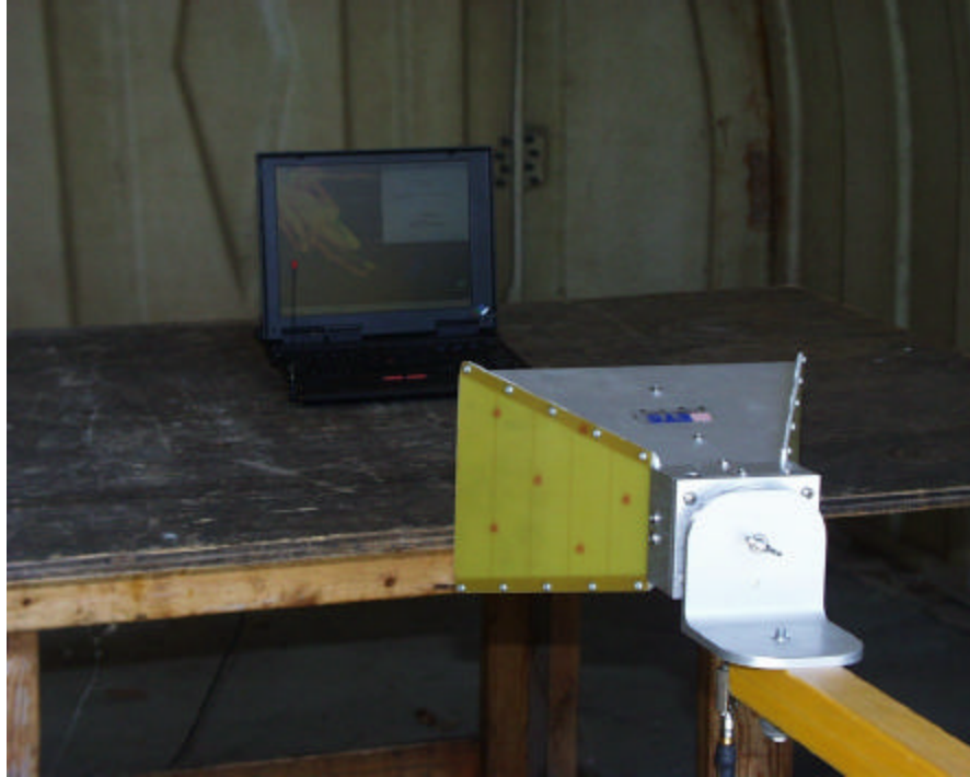
Above 1GHz Radiated Emission Setup
