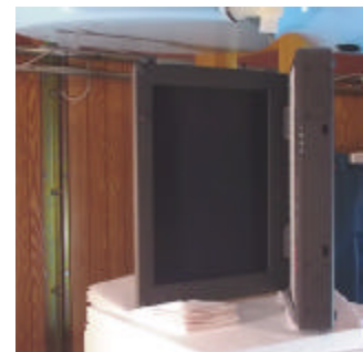
Body SAR Test Setup with 2.0cm separation distance
