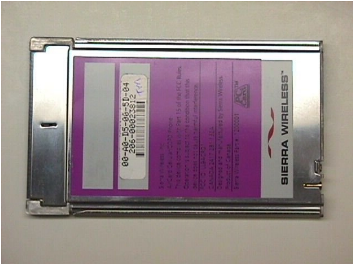
Figure 2: PCMCIA Card Bottom – Shows FCC label format and position
