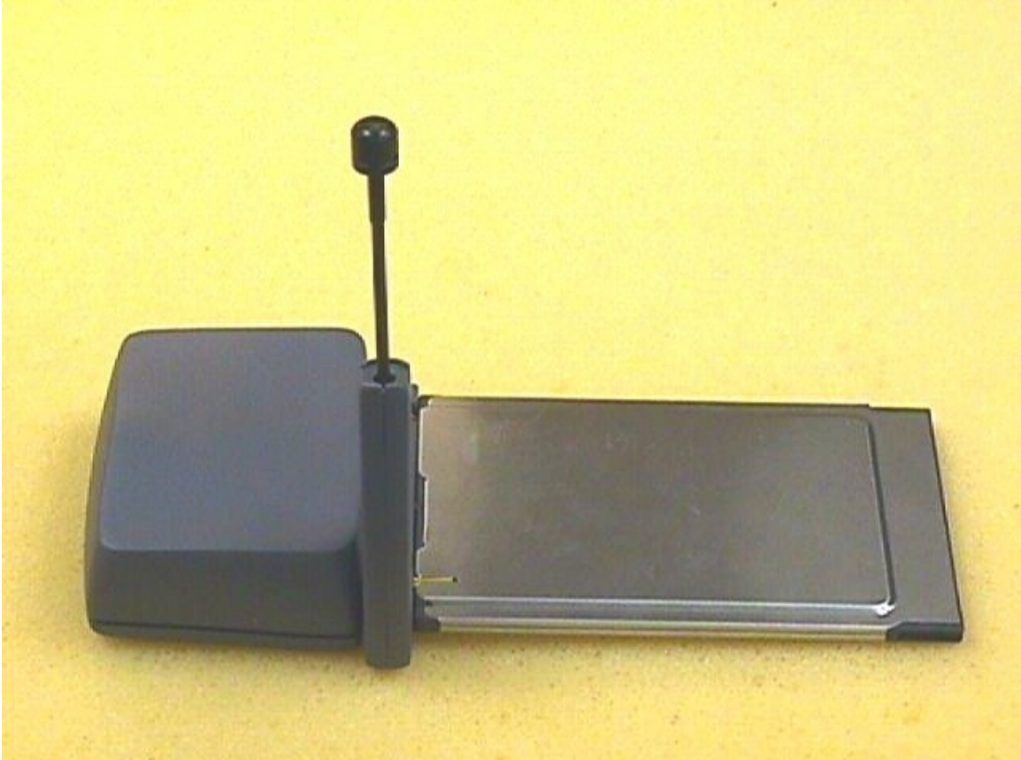
Figure 3: PCMCIA Card Prospective View – Shows antenna and battery bump attached
