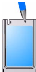
Figure 5-2: Ejecting the SIM card
