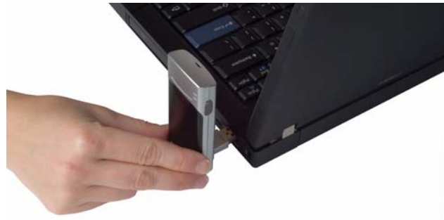
Figure 2-9: Correct way to insert the AirCard modem
