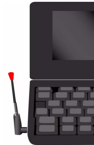
Figure 5-1: Proper positioning of the AirCard modem antenna for the AirCard 850/860 modems.
