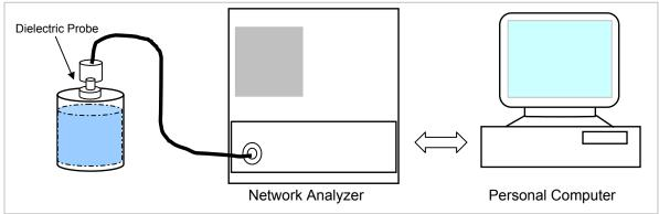
Set-up for liquid parameters check
