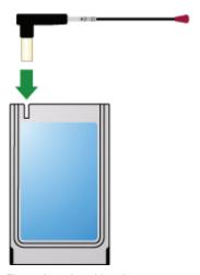
Figure 2-5: Attaching the antenna to the AirCard modem
