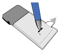
Figure 2-4: Ejecting the SIM card
