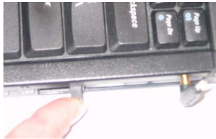
Figure 5-2: Ejecting the AirCard from its slot
