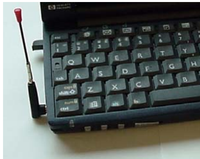
Figure 5-1: Proper positioning of the AirCard antenna
