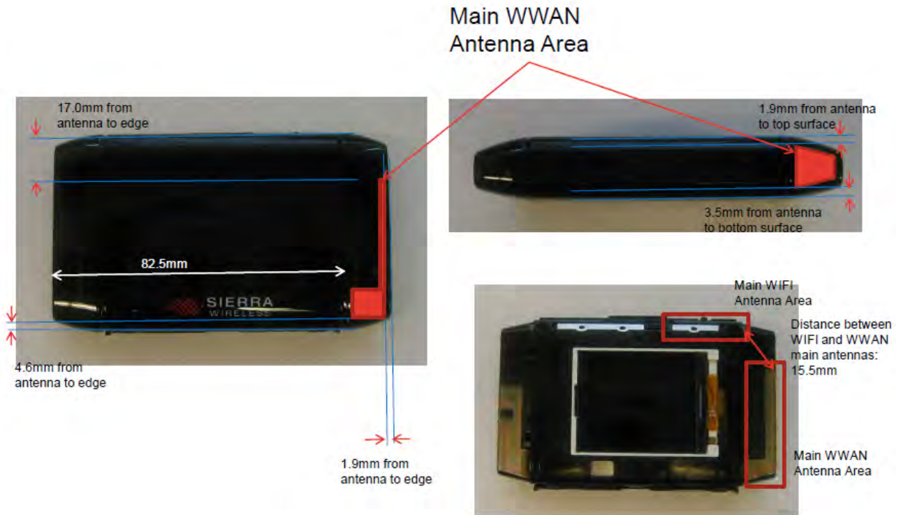
Fig.10 Antenna position of EUT (96.00 x 56.81 x 16.81 mm)
