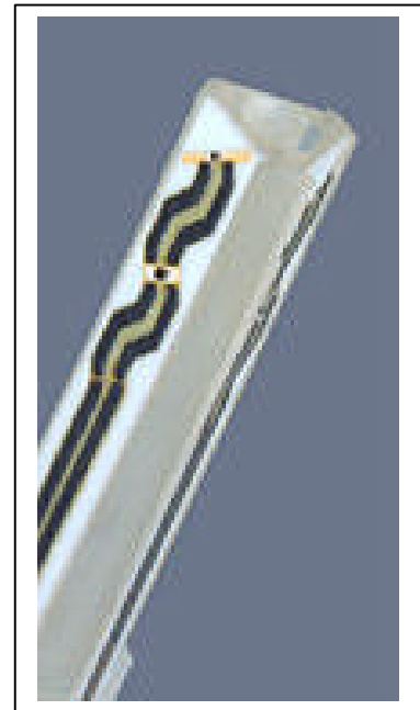
Inside view of ET3DV6 E-field Probe
