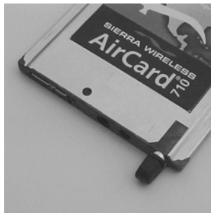
Figure 2-2: A SIM card properly inserted
