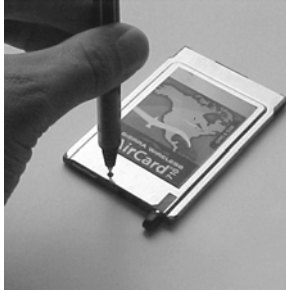
Figure 2-3: Positioning a pen to eject the SIM card
