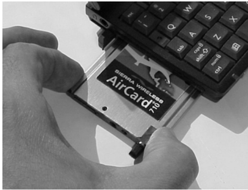
Figure 5-3: Removing the AirCard 710/750 PC Card from its slot
