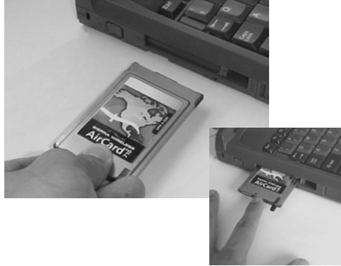
Figure 3-1: Inserting the AirCard 710/750 network card
