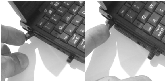
Figure 5-2: Ejecting the AirCard 710/750 PC Card from its slot
