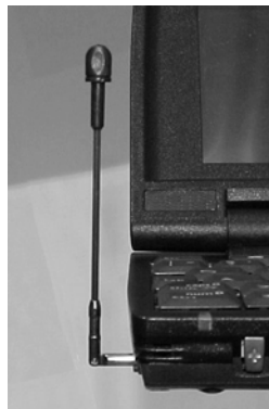
Figure 1-1: Proper positioning of the AirCard 710/750 antenna in a notebook
