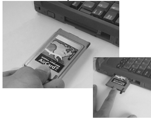
Figure 3-5: Inserting the AirCard 710/750 network card
