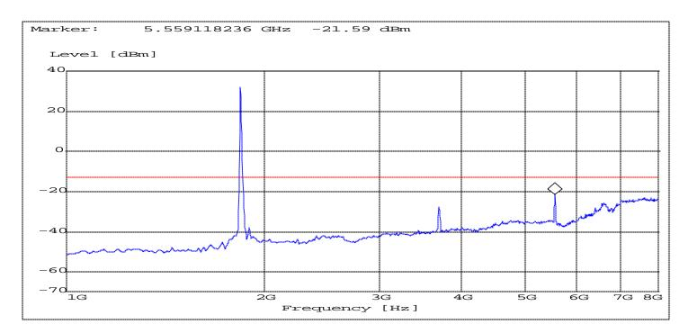
NOTE: Frequency resolution is not fine enough to show the exact frequency of the carrier, refer to plots under EIRP.
