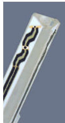
ET3DV6 E-Field Probe
