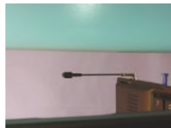
Body SAR Test Setup 2.0cm Separation Distance
