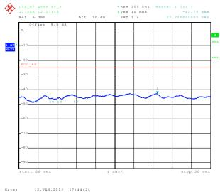
6.3.3.41 Out of Band Emissions at Antenna Terminals LTE B7, Mid channel, 2535.0 MHz, 10MHz BW, 50RB, QPSK, 30MHz to 1 GHz
