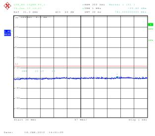
6.3.3.29 Out of Band Emissions at Antenna Terminals LTE B4, Low channel, 1720.0 MHz, 20MHz BW, 100RB, 16-QAM, 1 GHz to 10 GHz
