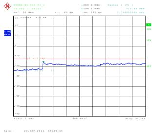
6.3.2.3 Out of Band Emissions at Antenna Terminals WCDMA, Middle channel, 836.4 MHz, 2 Hz to 1 GHz
