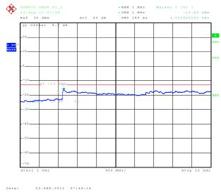
6.3.1.5 Out of Band Emissions at Antenna Terminals GMSK, High Channel, 848.8 MHz, 2 Hz to 1 GHz
