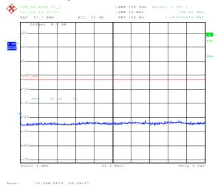
6.3.3.5 Out of Band Emissions at Antenna Terminals LTE B4, Mid channel, 1732.5 MHz, 10MHz BW, 50RB, QPSK, 1 GHz to 10 GHz
