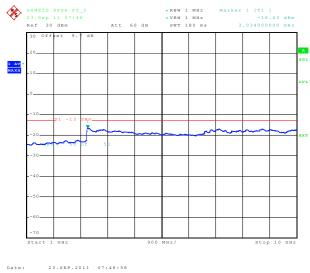
6.3.1.9 Out of Band Emissions at Antenna Terminals 8-PSK, Mid Channel, 836.6 MHz, 2 Hz to 1 GHz
