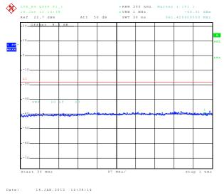
6.3.3.23 Out of Band Emissions at Antenna Terminals LTE B4, Mid channel, 1732.5 MHz, 20MHz BW, 100RB, QPSK, 1 GHz to 10 GHz
