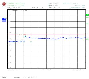
6.3.1.13 Out of Band Emissions at Antenna Terminals GMSK, Low channel, 1850.2 MHz, 2 Hz to 1 GHz
