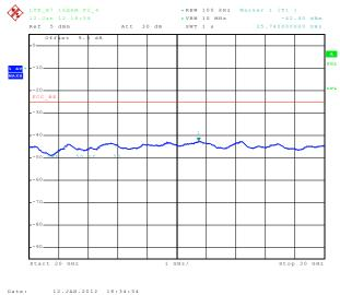
6.3.3.61 Out of Band Emissions at Antenna Terminals LTE B7, Low channel, 2510.0 MHz, 20MHz BW, 100RB, QPSK, 30MHz to 1 GHz
