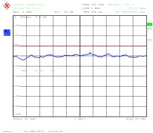
6.3.3.77 Out of Band Emissions at Antenna Terminals LTE B7, Mid channel, 2535.0 MHz, 20MHz BW, 100RB, 16QAM, 30MHz to 1 GHz
