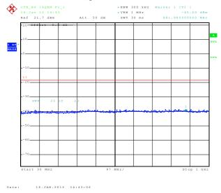
6.3.3.35 Out of Band Emissions at Antenna Terminals LTE B4, High channel, 1745.0 MHz, 20MHz BW, 100RB, 16-QAM, 1 GHz to 10 GHz
