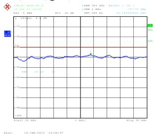
6.3.3.69 Out of Band Emissions at Antenna Terminals LTE B7, High channel, 2560.0 MHz, 20MHz BW, 100RB, QPSK, 30MHz to 1 GHz
