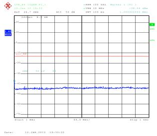
6.3.3.17 Out of Band Emissions at Antenna Terminals LTE B4, High channel, 1750.0 MHz, 10MHz BW, 50RB, 16-QAM, 1 GHz to 10 GHz
