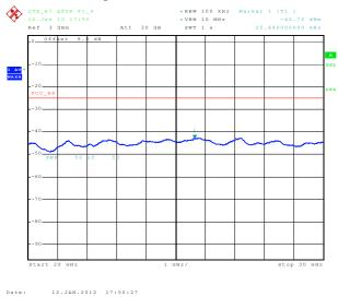
6.3.3.45 Out of Band Emissions at Antenna Terminals LTE B7, High channel, 2565.0 MHz, 10MHz BW, 50RB, QPSK, 30MHz to 1 GHz
