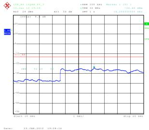
6.3.3.13 Out of Band Emissions at Antenna Terminals LTE B4, Mid channel, 1732.5 MHz, 10MHz BW, 50RB, 16-QAM, 30MHz to 1 GHz
