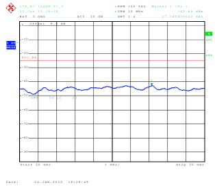
6.3.3.57 Out of Band Emissions at Antenna Terminals LTE B7, High channel, 2565.0 MHz, 10MHz BW, 50RB, 16QAM, 30MHz to 1 GHz
