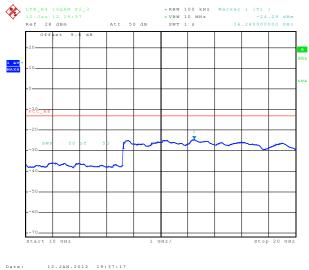
6.3.3.19 Out of Band Emissions at Antenna Terminals LTE B4, Low channel, 1720.0 MHz, 20MHz BW, 100RB, QPSK, 30MHz to 1 GHz
