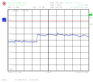
6.3.3.37 Out of Band Emissions at Antenna Terminals LTE B7, Low channel, 2505.0 MHz, 10MHz BW, 50RB, QPSK, 30MHz to 1 GHz
