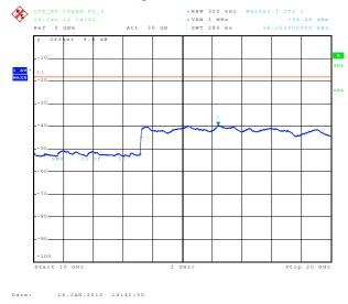
6.3.3.31 Out of Band Emissions at Antenna Terminals LTE B4, Mid channel, 1732.5 MHz, 20MHz BW, 100RB, 16-QAM, 30MHz to 1 GHz
