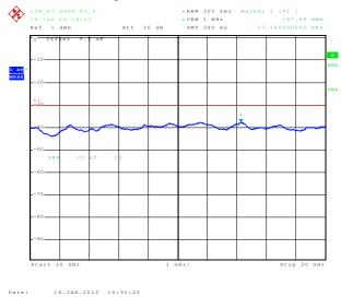
6.3.3.73 Out of Band Emissions at Antenna Terminals LTE B7, Low channel, 2510.0 MHz, 20MHz BW, 100RB, 16QAM, 30MHz to 1 GHz
