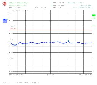
6.3.3.53 Out of Band Emissions at Antenna Terminals LTE B7, Mid channel, 2535.0 MHz, 10MHz BW, 50RB, 16QAM, 30MHz to 1 GHz
