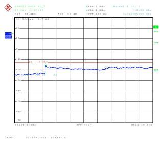
6.3.1.3 Out of Band Emissions at Antenna Terminals GMSK, Mid Channel, 836.6 MHz, 2 Hz to 1 GHz
