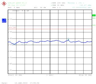
6.3.3.49 Out of Band Emissions at Antenna Terminals LTE B7, Low channel, 2505.0 MHz, 10MHz BW, 50RB, 16QAM, 30MHz to 1 GHz
