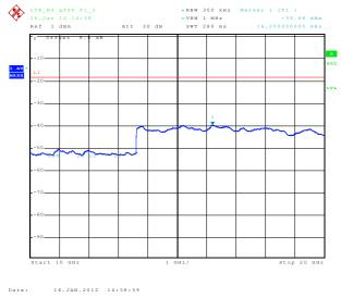
6.3.3.25 Out of Band Emissions at Antenna Terminals LTE B4, High channel, 1745.0 MHz, 20MHz BW, 100RB, QPSK, 30MHz to 1 GHz
