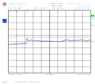
6.3.1.7 Out of Band Emissions at Antenna Terminals 8-PSK, Low channel, 824.200 MHz,2 Hz to 1 GHz
