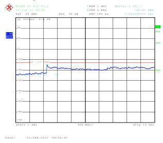
6.3.2.5 Out of Band Emissions at Antenna Terminals WCDMA, High Channel, 846.6 MHz, 2 Hz to 1 GHz
