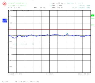
6.3.3.65 Out of Band Emissions at Antenna Terminals LTE B7, Mid channel, 2535.0 MHz, 20MHz BW, 100RB, QPSK, 30MHz to 1 GHz
