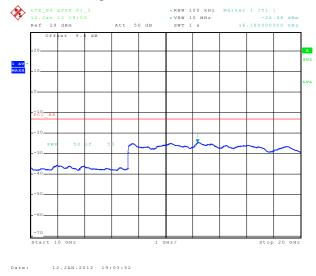
6.3.3.7 Out of Band Emissions at Antenna Terminals LTE B4, High channel, 1750.0 MHz, 10MHz BW, 50RB, QPSK, 30MHz to 1 GHz
