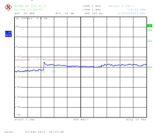
6.3.2.7 Out of Band Emissions at Antenna Terminals WCDMA, Low channel, 1852.4 MHz, 2 Hz to 1 GHz
