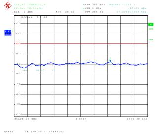
6.3.3.81 Out of Band Emissions at Antenna Terminals LTE B7, High channel, 2560.0 MHz, 20MHz BW, 100RB, 16QAM, 30MHz to 1 GHz
