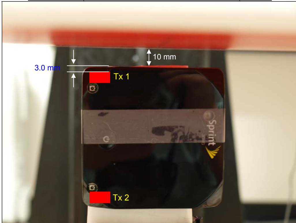
Seup photo for TX1 Antenna with 10 mm separation distance from side of the EUT to phantom
