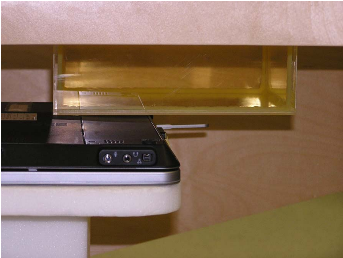
Photo 2. Lap B Main WWAN and WLAN Antennas Position
