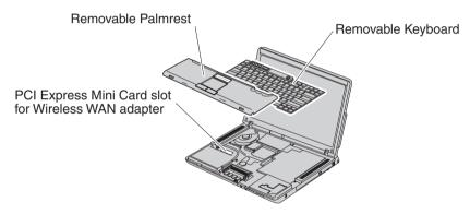
**Attention:** The ThinkPad Z61 Series computer contains an authentication mechanism If you install an unauthorized wireless WAN Mini PCI Express Card that is not approved for use in the ThinkPad Z61 Series computer, the computer will not start, but only displays an error message and emits beeps.
