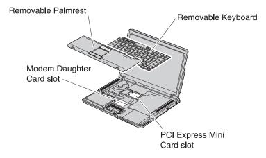
**Attention:** The ThinkPad Z60t Series computer contains an authentication mechanism You can install or remove each wireless feature by yourself. If you install an unauthorized wireless adapter that is not approved for use in the ThinkPad Z60t Series computer, the computer will not start, but only displays an error message and emits beeps.
