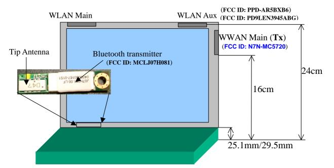
Figure-2 Antenna assembly of X60 series
