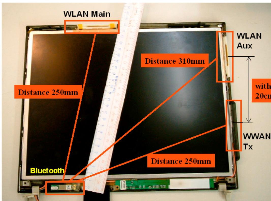
Figure-2 Antenna assembly of X60 series
