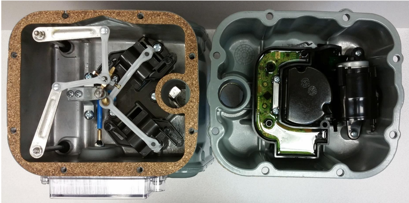
The meter top is rotated 180 degrees away from the meter body. There are no electronic components in the meter body in the left half of the picture.
