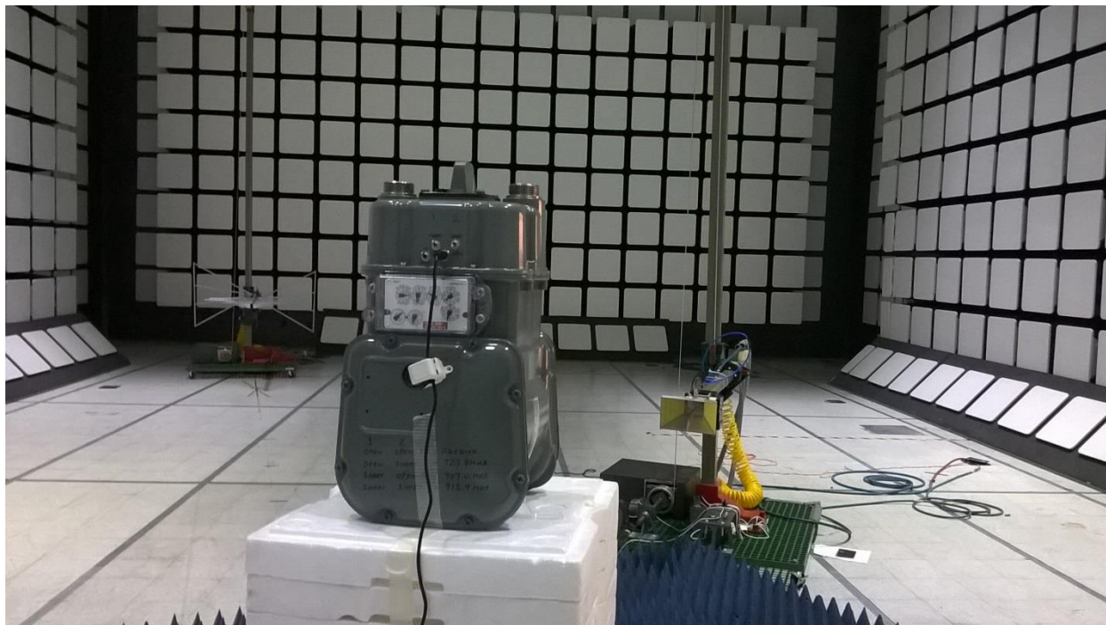
Figure 5 - Radiated Emissions Test Setup, 1 – 10 GHz
