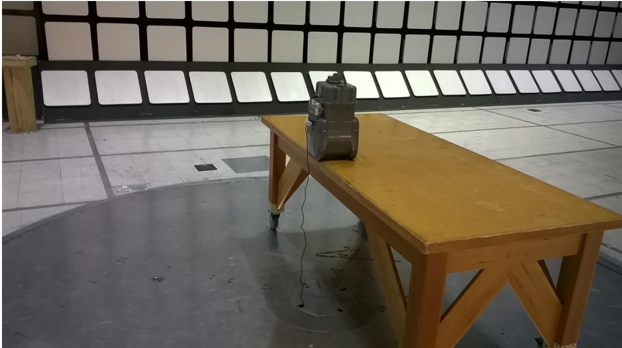
Figure 2 - Radiated Emissions Test Setup, 30Mhz - 1GHz
