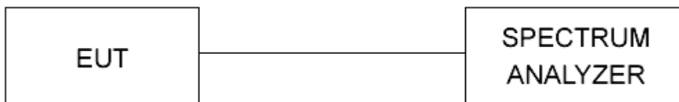
Figure 10 - Bandwidth Measurements Test Setup
