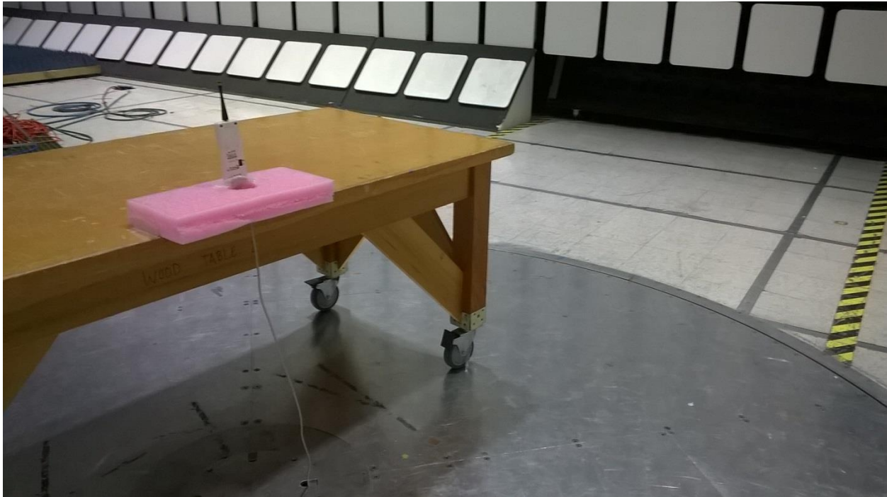
Figure 3 - 30MHz - 1GHz, Antenna = ANT-919-CW-QW, Z-axis up, Vertical Antenna
