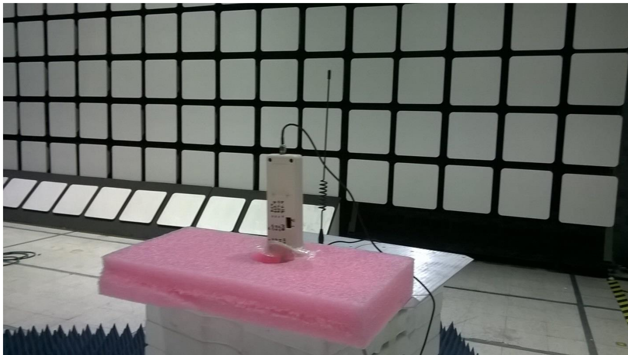
Figure 7 - 1GHz – 10GHz, Antenna = ANT-ELE-S01-005, Z-axis up, Vertical Antenna
