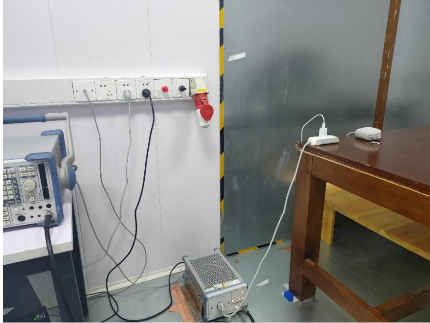
Conducted Emissions at AC Power Line (150kHz-30MHz)
