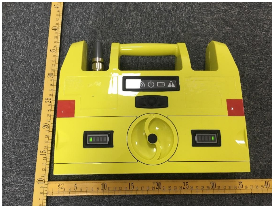
Wireless Repeater Node (Model: W-WRN-000)
