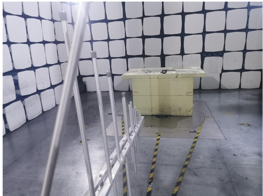
Radiation Emission Test Setup (30MHz to 1GHz)
