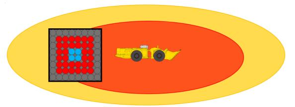
The exiting personnel's tag vibrates, emits an audible alarm, and its LED flashes red, which continues while the tag remains in the Danger zone.
