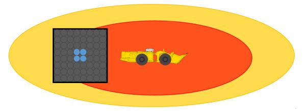
2. Personnel carrying a tag enters the Warning zone and yellow LEDs flash on the display panel and the audible alarm sounds, which continues while the tag remains in the Warning zone. The blue LEDs remain since the operator is in the cabin.
