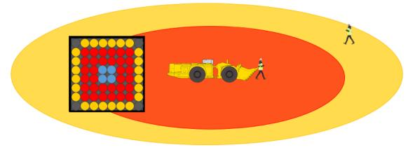
The second person's tag vibrates, emit an audible alarm, and its LED will flash yellow, which continues while the tag remains in the Warning zone.
