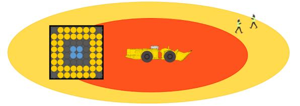
The first person's tag vibrates, emits an audible alarm, and its LED flashes yellow, which continues while the tag remains in the Warning zone.
