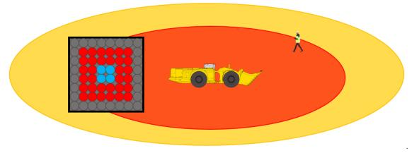
The approaching personnel tag vibrates, emits an audible alarm, and its LED flashes red, which continues while the tag remains in the Danger zone.
