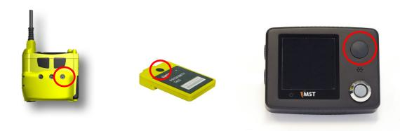
Pressing the suppression button on a personnel tag or ICCL embedded tag will suppress the vibration and the audible alarm; the LED will also stop flashing and illuminate permanently. Suppression of the alarms allows personnel to concentrate on taking corrective action. This suppression is only temporary and all the alarm behaviours will resume after a user configurable time span.
