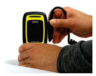
**4.** Use a flathead screwdriver to tighten the screw on the RSM jack to the MinePhone.
