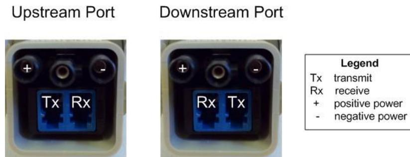
Figure 4: Fibre orientation of Upstream and Downstream ports
