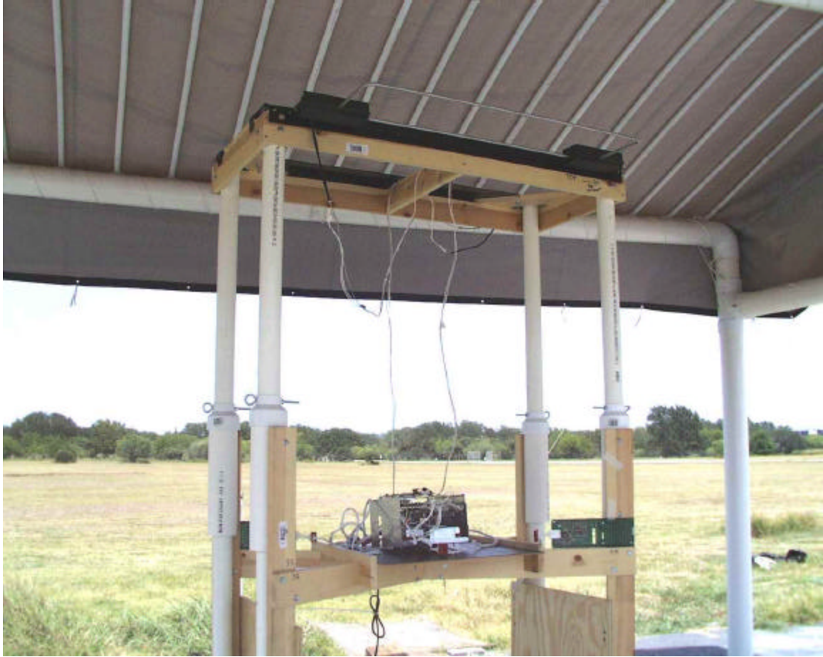
Radiated Emissions OATS Test Setup – Encore Configuration
