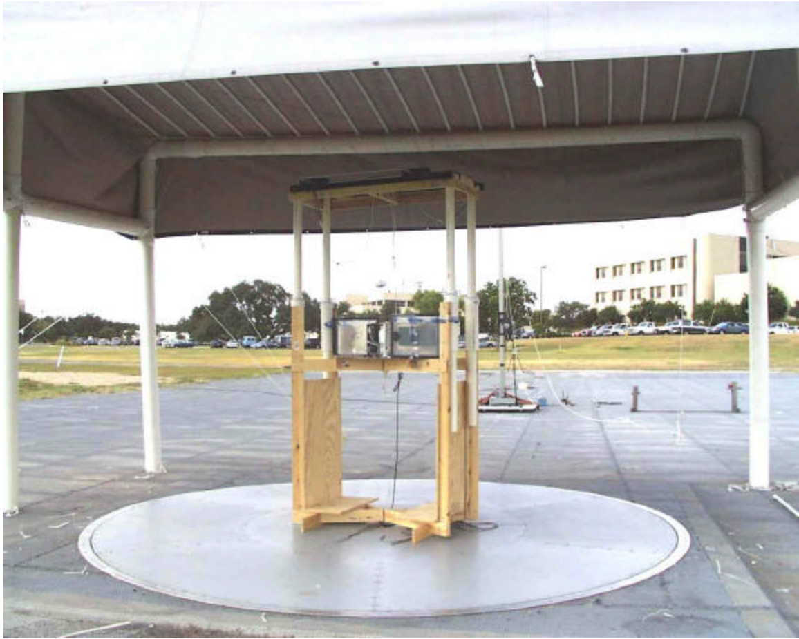
Radiated Emissions OATS Test Setup – Advantage Configuration
