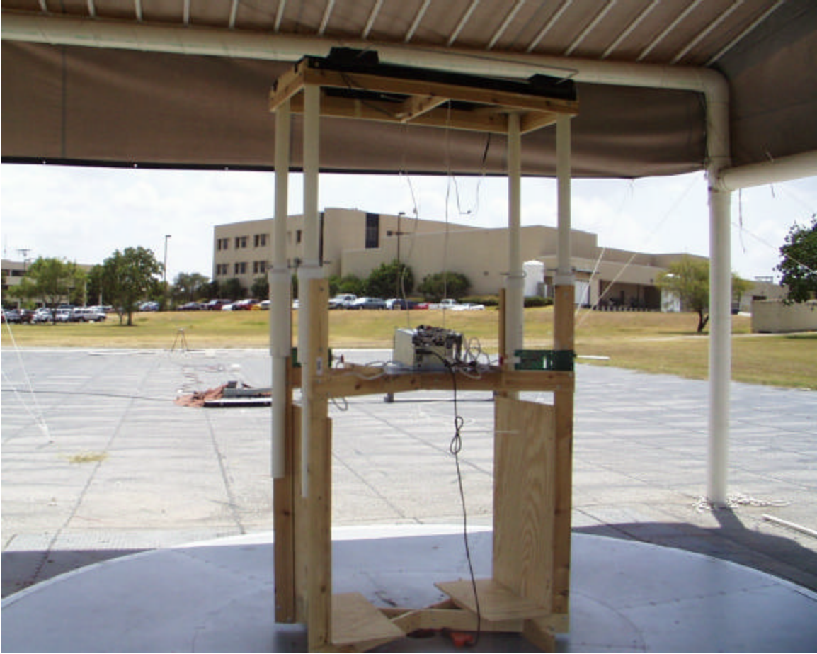
Radiated Emissions OATS Test Setup – Encore Configuration
