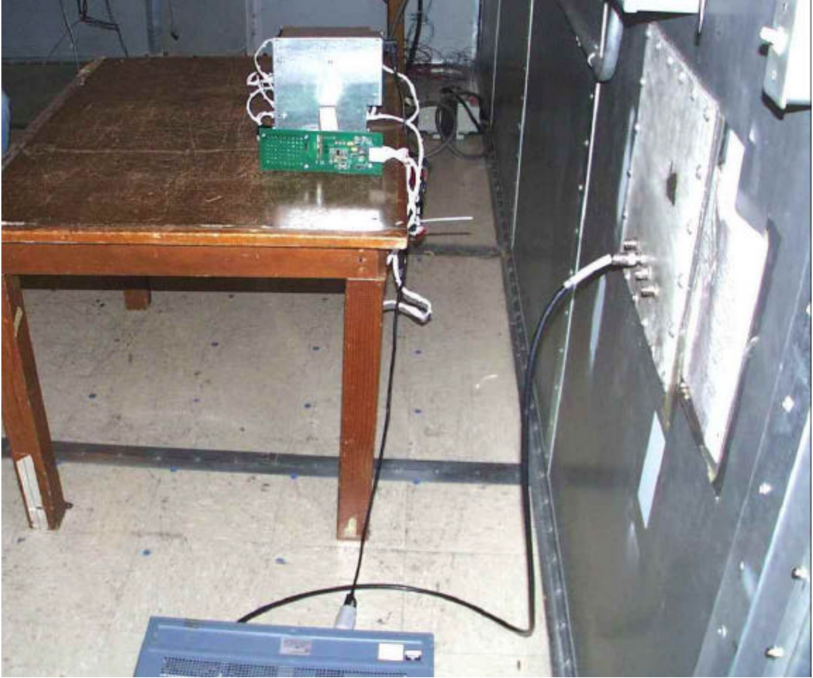
Conducted Emissions Test Setup – Encore Configuration
