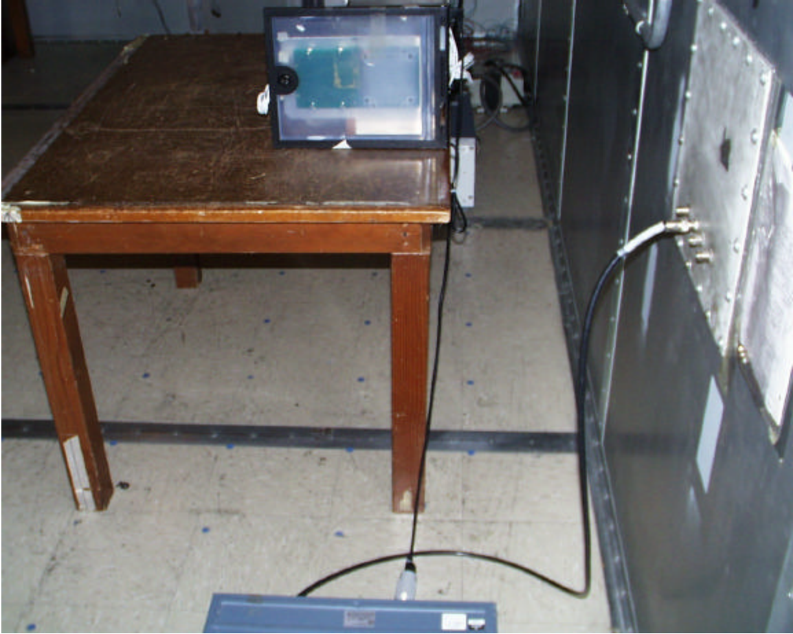
Conducted Emissions Test Setup – Advantage Configuration
