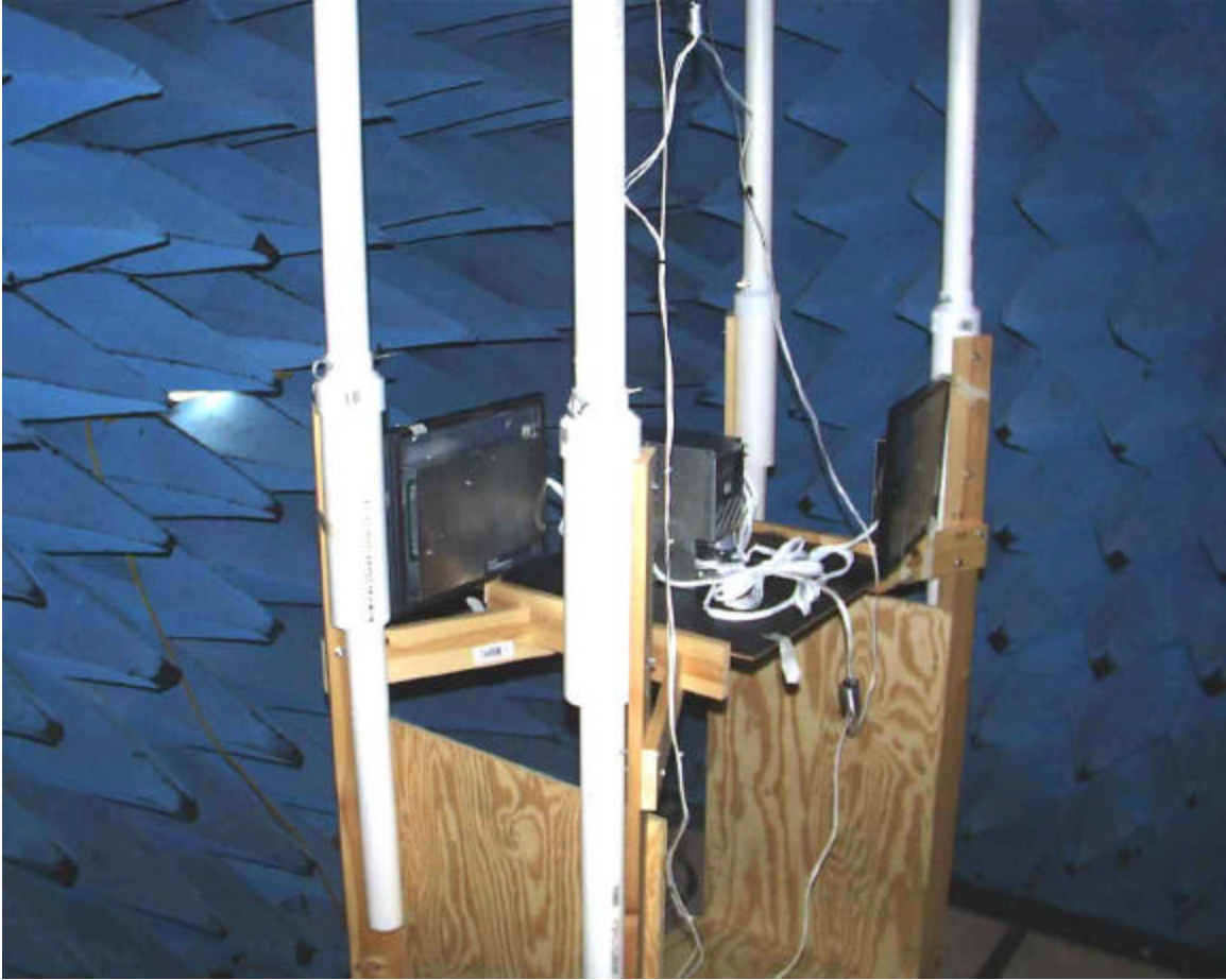
Radiated Emissions Pre-scan (Anechoic) Test Setup – Advantage Configuration
