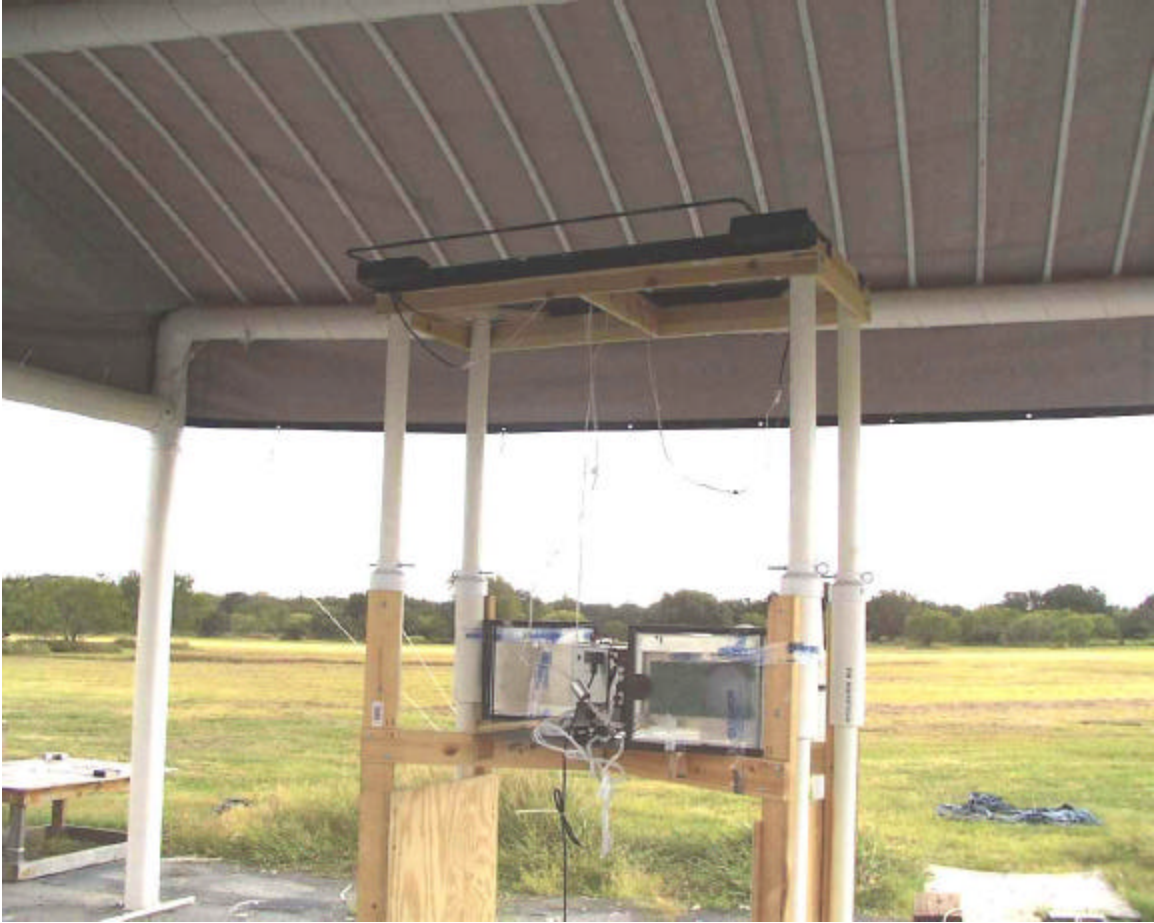
Radiated Emissions OATS Test Setup – Advantage Configuration
