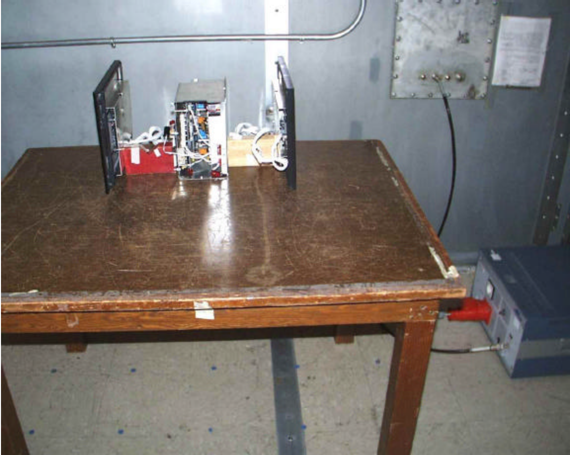
Conducted Emissions Test Setup – Advantage Configuration
