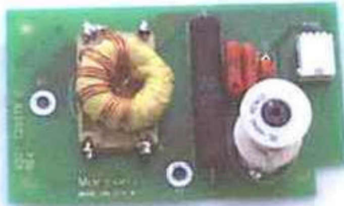
Encore Overhead Antenna (Low Frequency) Tuning Board (Frontside)
