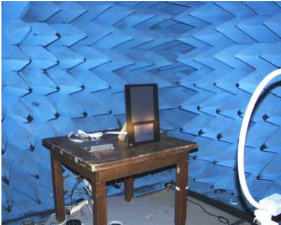
Radiated Emissions Pre-scan (Anechoic) Test Setup
