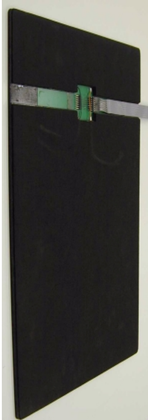
N6SMRIR11 Marconi Commerce Systems - Mat Reader (BackView - shows ribbon cable connection)
